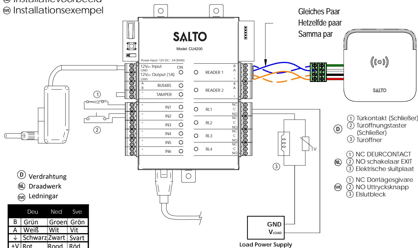
SALTO recommends always using an external power supply to operate the load.
