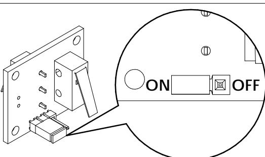
Note: To override the wall tamper, place the jumper in OFF position.
