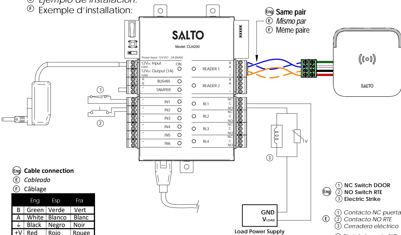
SALTO recommends always using an external power supply to operate the load.
