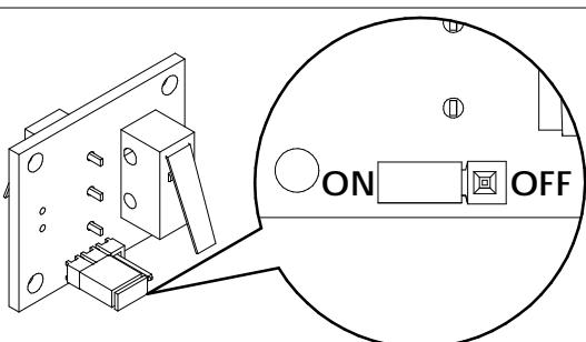
Note: To override the wall tamper, place the jumper in OFF position.
