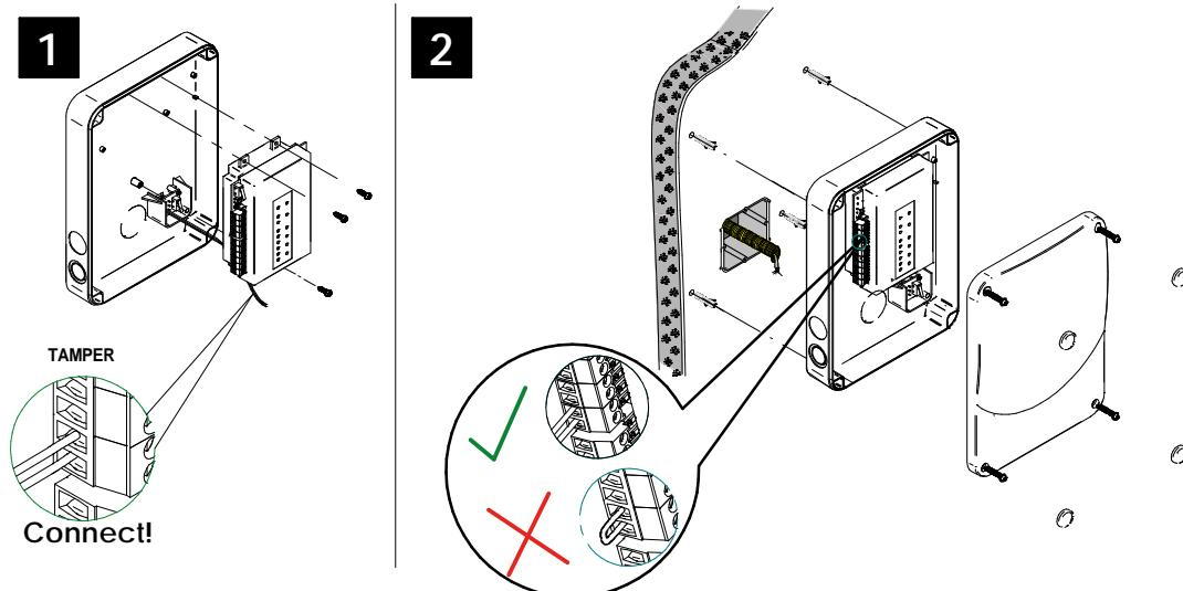
Note: Follow the same connection model, using the CU tamper input, when using a third party electric box equipped with a tamper opening detection.
